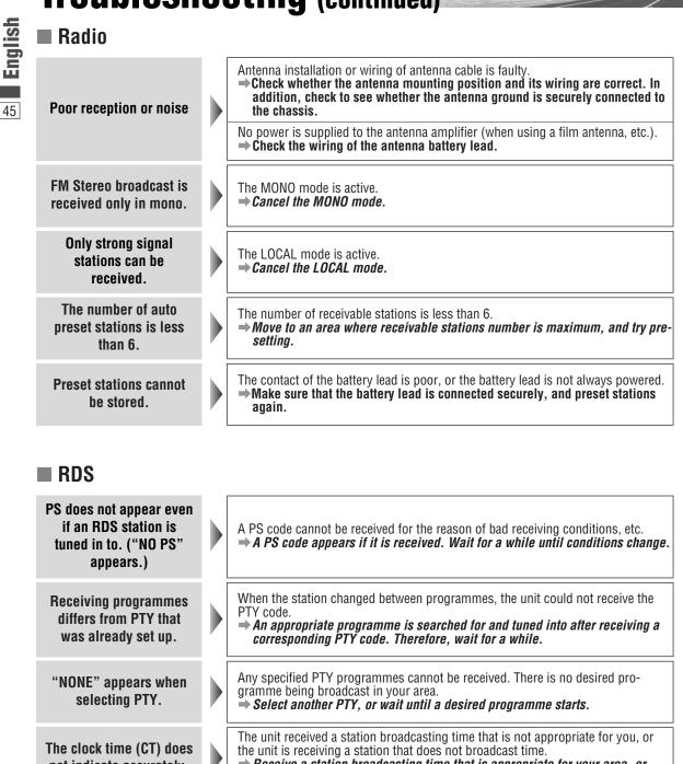
Receive a station broadcasting time that is appropriate for your area, or adjust CT manually.
